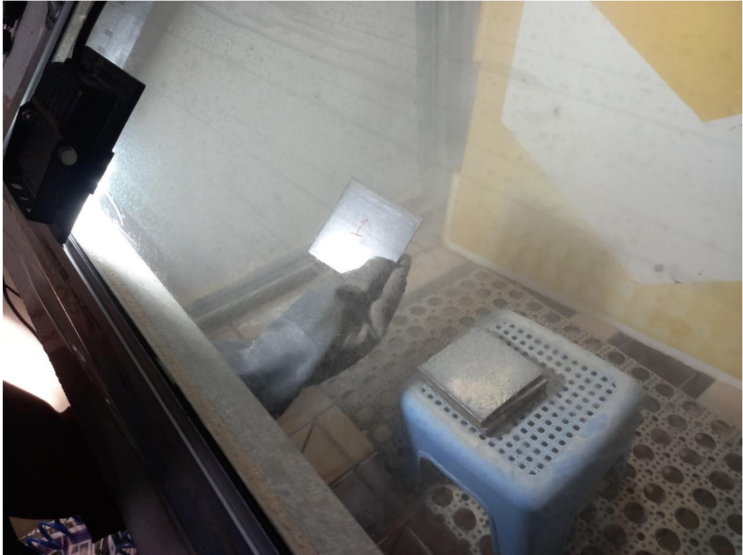
Lampiran 2 Gambar Proses Sandblasting
