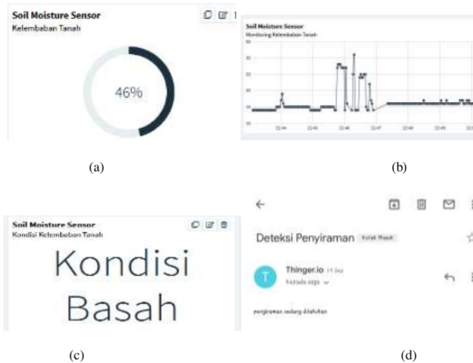
Figure 8. Monitoring soil moisture (a) water content value, (b) soil (c) soil condition (d) notification of watering process
