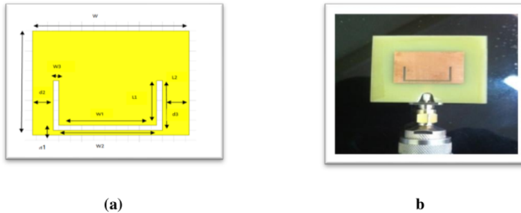
Figure 5. The geometry of Patch Antenna`
